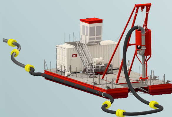
Vertical deployment type – for dredging loosely compacted soil
